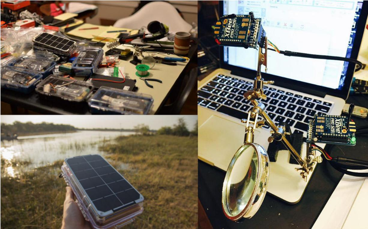
Each of the nodes consist of an [Arduino](#), [XBee](#), and multiple sensors. The XBee ZigBee network makes it possible to connect over long distances since data packets can hop between neighboring nodes until they reach the central coordinator. For power, the remote nodes rely on a solar panel and a 6600 mAh battery.
